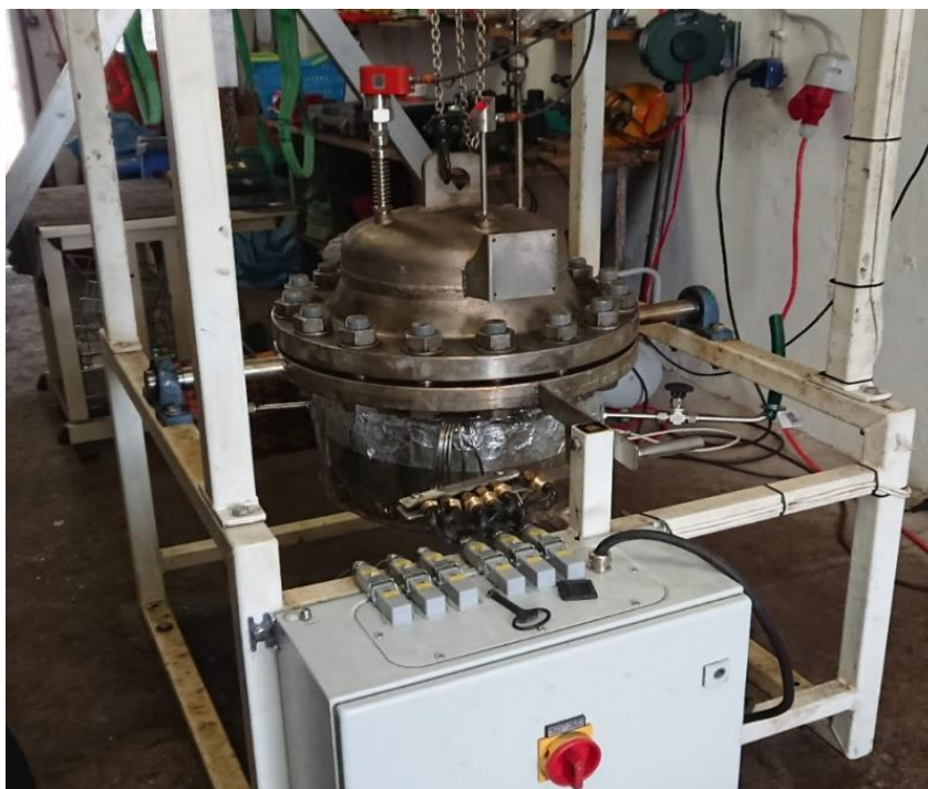
Figure 4. Biochar production in lab scale. Source: Presentation by Timo Garrels, KS-VTCTech GmbH, available at https://www.coastal-biogas.eu/events/conference-germany/
