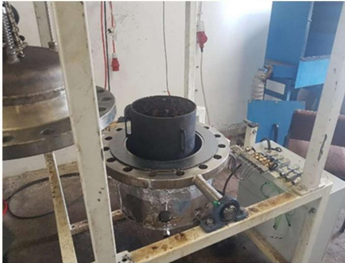
Reactor with open pressure vessel
