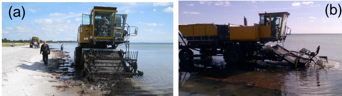
Figure 14: The prototype of seaweed harvester: (a) – front view; (b) – side view
