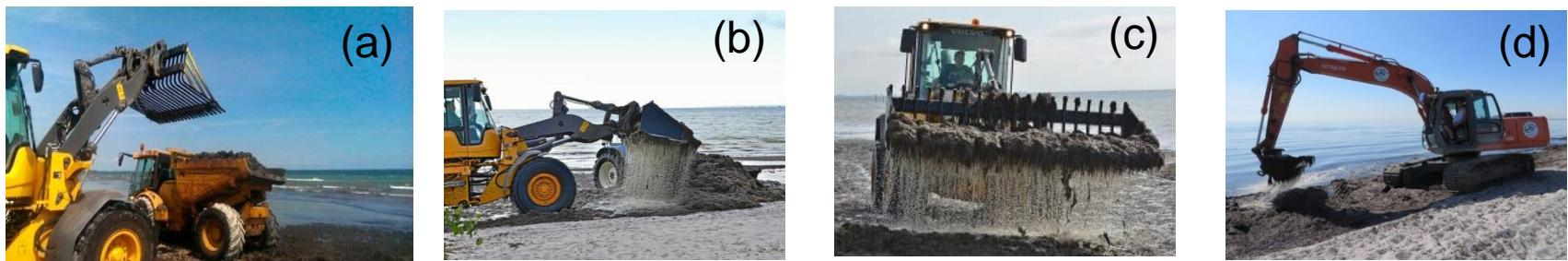
Figure 15: (a-c) – loader tractor, (d) - backhoe with a big shovel in front, rinsing of the sandy seaweed
