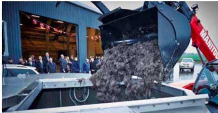
Figure 18: Seaweed supply in a receiving tank wth a stirrer
