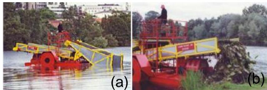
**Figure 5:** Pontoon machine (Limnocombine): (a) – side view; (b) – backside view
