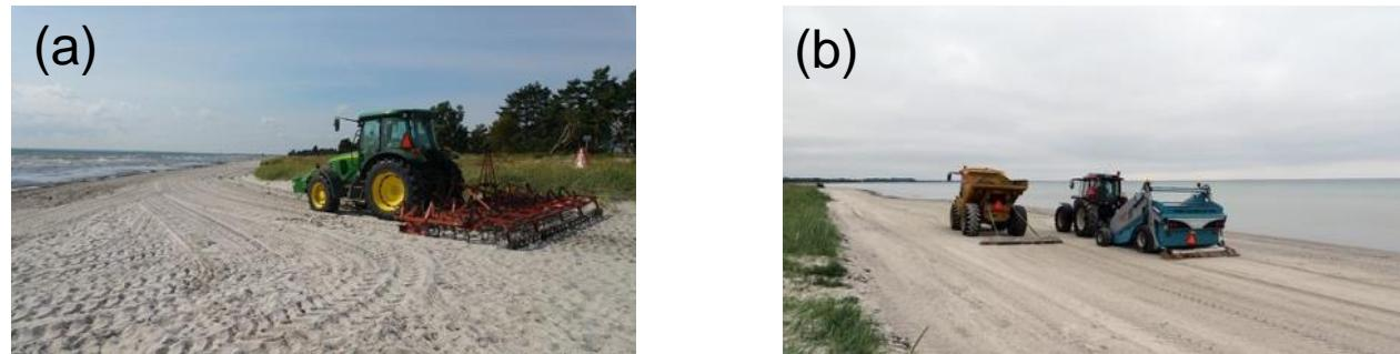
**Figure 17:** (a) – a tractor (b) – a dump truck and a seaweed collecting machine clear the ruts of seaweed
