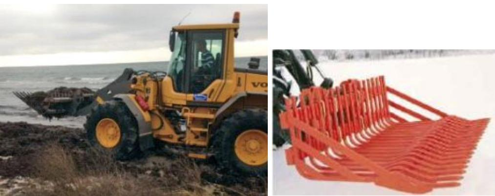
**Figure 3:** A wheel loader with a pitchfork or bucket
