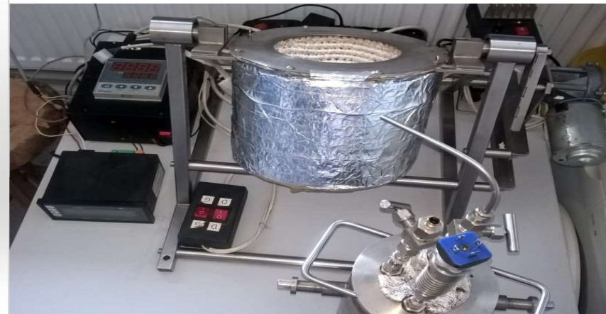
System for thermal treatment of biomass (1) steam generator, (2) autoclave for hydrothermal lysis, (3) balance for measuring steam consumption, (4) control system; (5) steam connection.
